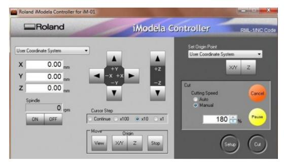
From the **Cut** panel on the right you can click on **manual**, change the speed in percentage. If set to manual you can also change during the milling phase.
