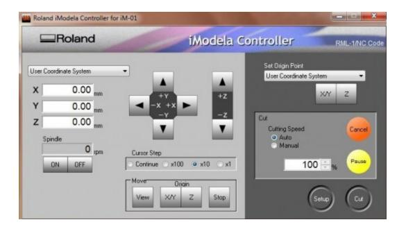
clicking on the various alternatives of the Cursor Step (**continuous - x 100 - x 10 - x 1**) you choose how many steps the spindle moves on different axes, each step is 0.01mm
