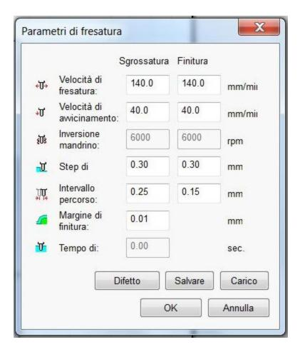
In this way the drill will make two passes to reduce vibration and efforts on the spindle. The speed of rotation (**reversing spindle**) can not be changed from here, will be changed by the controller.
