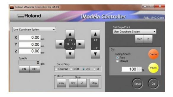
clicking on the various alternatives of the **Cursor Step (continuous - x 100 - x 1)** you choose the number of steps of how much move the spindle on different axes, <u>each step is 0.01mm</u>.
