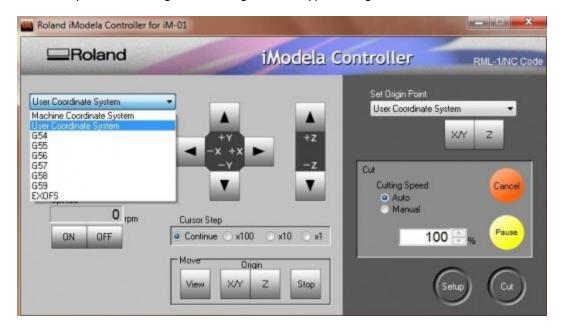
Set **User Coordinate System** in both pull-down menu (upper left and upper right)
