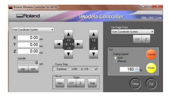
From the **Cut** the panel on the right you can, by clicking on **manual**, change the speed in percentage. If set to manual you can also change during the milling phase
